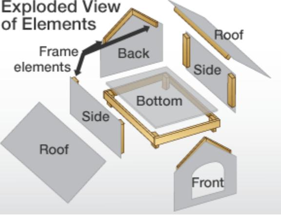
**Step 1:** Lay out the panels on the back of the siding as shown in the drawing. Then, carefully cut out the panels on the lines. Cut the entry hole only large enough to allow your dog easy access.
